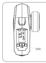
CH3 key setting function: CH3 key can automatically switch between positive and negative output self-locking or non self-locking. Long press CH3 key buzzer to give a sound, indicating successful switching. (Factory default self-locking)
