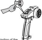
The LED on the receiver will now remain solid to indicate successful binding of the transmitter and receiver.
