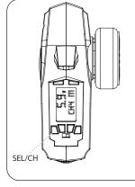
Restore factory settings: In the startup state, long press and hold the "SEL/CH" button, the buzzer will beep once, the LCD screen will go out, and then restart.
